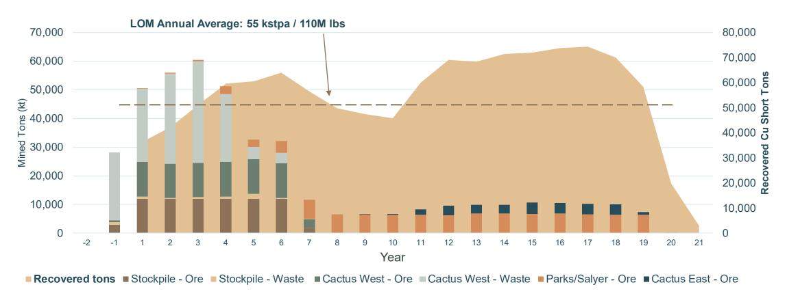
The mining schedule reflects a layered mining plan targeted at early production with low capex, maximizing project returns. Initial plant capacity is designed at 30 ktpa with expansion to 60 ktpa concurrent with underground mining in full ramp up by year 7 of the project start-up.
